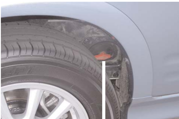
Manual Hydrogen Shut-Off Valve
