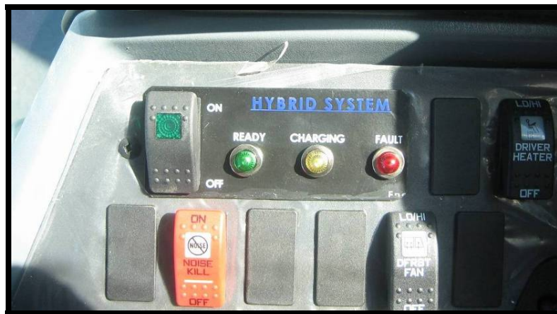
Figure 4.1: Hybrid System – Driver interface panel
